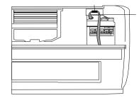
•Ground wire: Remove the grounding screw out of the electric bracket, cover the grounding wire end onto the grounding screw and screw it into the grounding hole.
